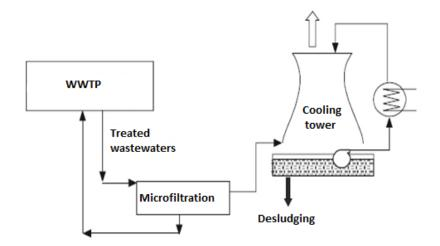
Wastewater treated at urban WWTP still need further treatment. In spite that physical and chemical parameters of delivered waste water are not constant, the product after microfiltration process meets all requirements for cooling medium.
